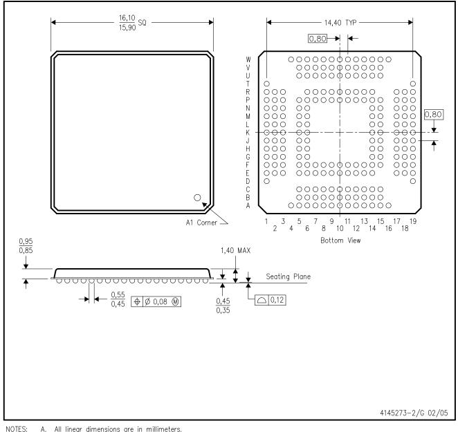
A. All linear dimensions are in millimeters.
